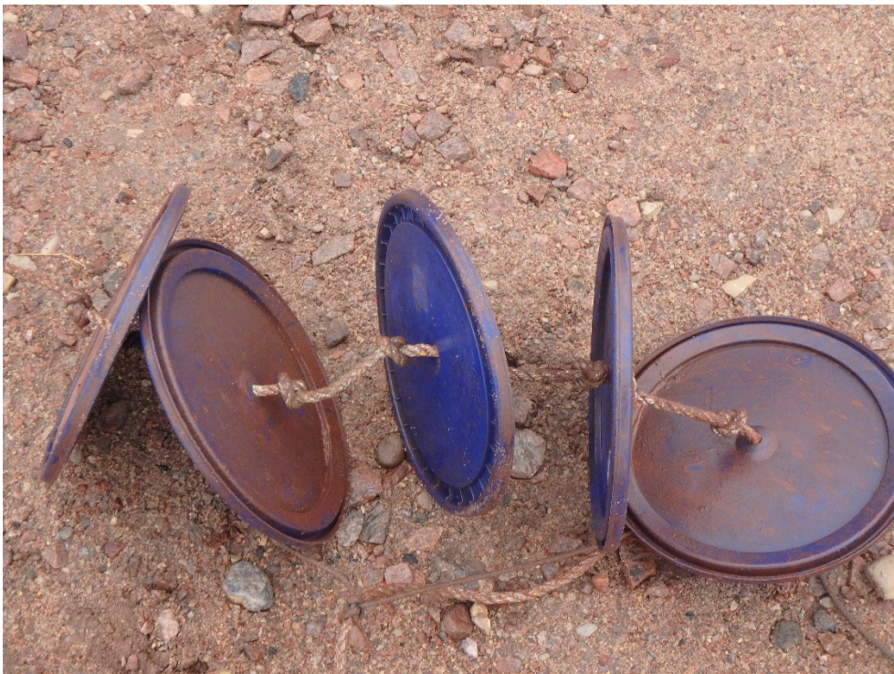
Photo 6: Settlement plates from western side of Milne Port Ore Dock (SBWO-1) found washed up on shore in August 2019
