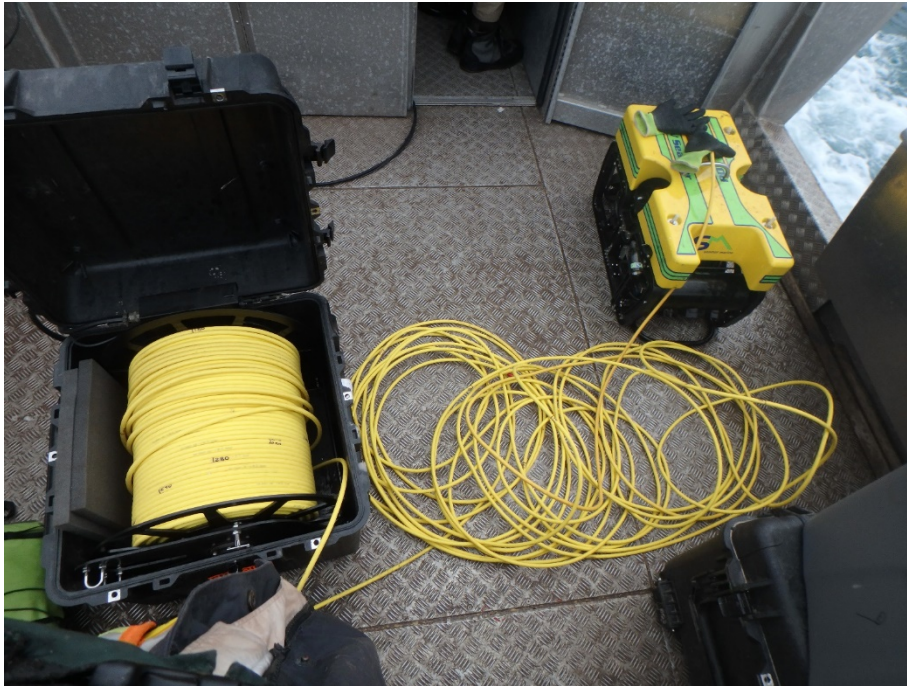
Figure 1: Photograph showing set-up of Seamor Chinook 300F ROV on deck of field vessel used to undertake underwater video surveys of offset habitat along Milne Port Ore Dock (August 2019).
