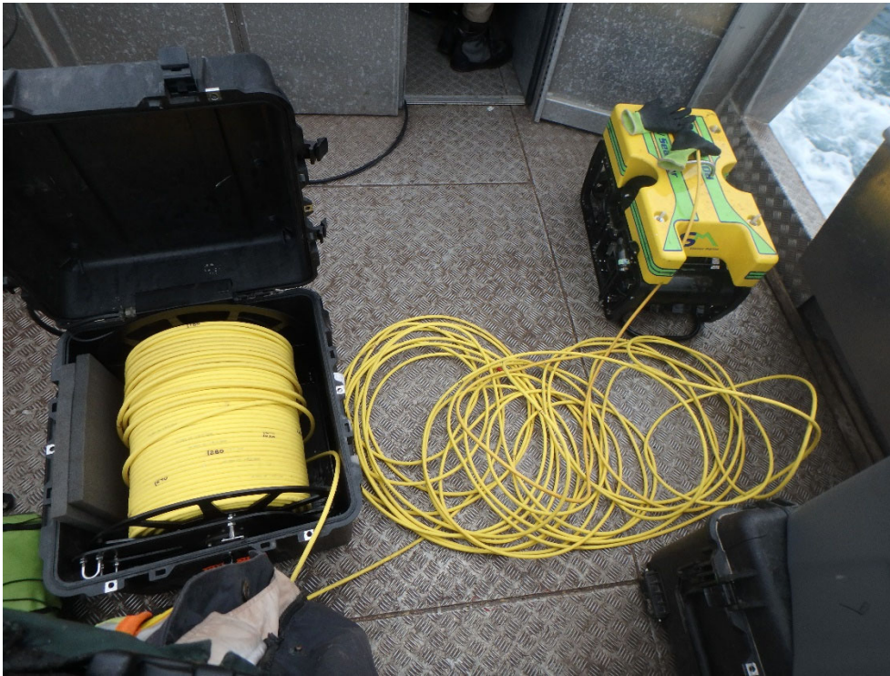
Photo 1: Seamor Chinook 300F ROV video system used to undertake underwater video surveys of offset habitat along Milne Port Ore Dock in August 2019
