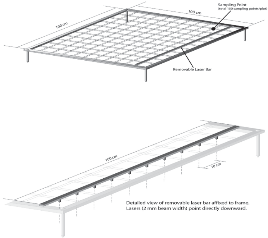
Figure 15 Illustration of the point quadrat frame used to measure percent plant cover.
