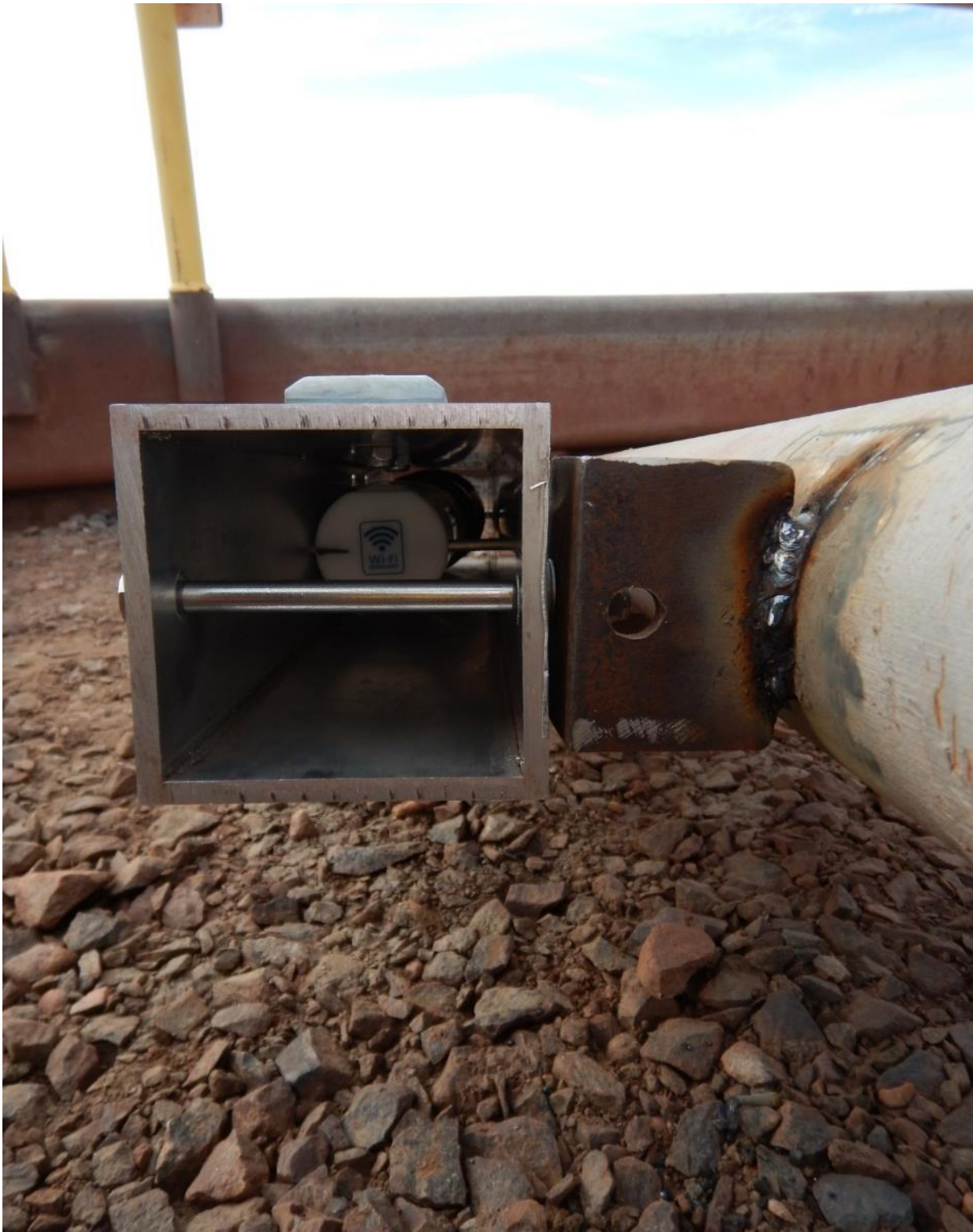
Figure 4: Hardware attaching aluminum tube to L brackets and view of the tide gauge mounted in the tube. Arrow shows location of the 1/4" bolt that should pass through the end cap of the tide gauge.
