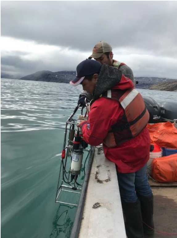
Photograph 15: Field team deploying CTD Seabird at one of the Ragged Island station locations on 8 August 2018.
