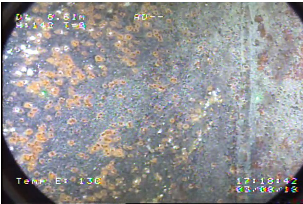
Figure 4-33: Arkadia ship hull with encrusting barnacles from ROV footage.
