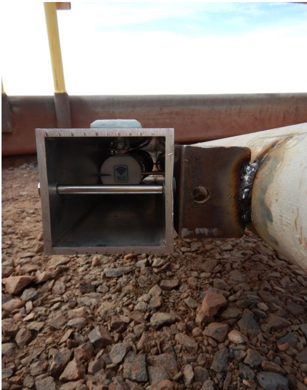
Figure 3: Hardware attaching aluminum tube to L brackets and view of the tide gauge mounted in the tube. Arrow shows location of the 1/4" bolt that should pass through the end cap of the tide gauge.
