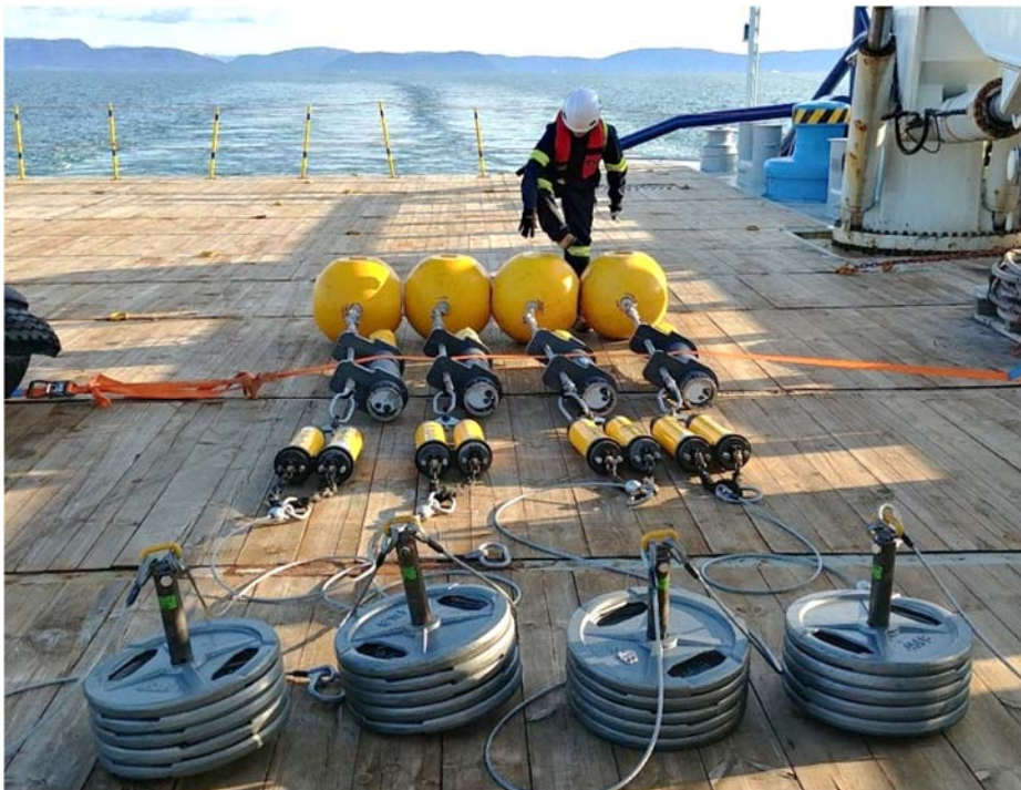
Figure 2. The Autonomous Multichannel Acoustic Recorder – Generation 3 (AMAR G3; JASCO) positioned in the middle of the mooring. AMARs were used to measure underwater sound.
