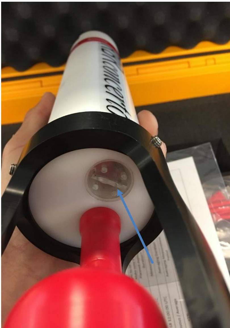
Figure 6: Pressure sensor location, shown by the arrow, on the downward facing end of the tide gauge
