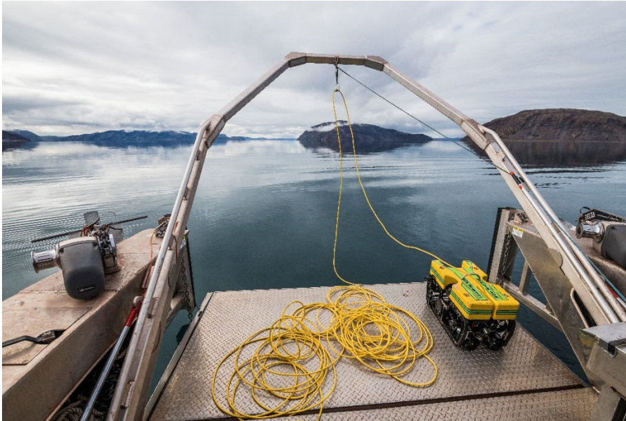
Figure 1: Photograph showing set-up of Seamor Chinook 300F ROV on deck of the research vessel used to undertake underwater video surveys at Milne Port (August 2020). Source: Jeff Reynolds 2020.
