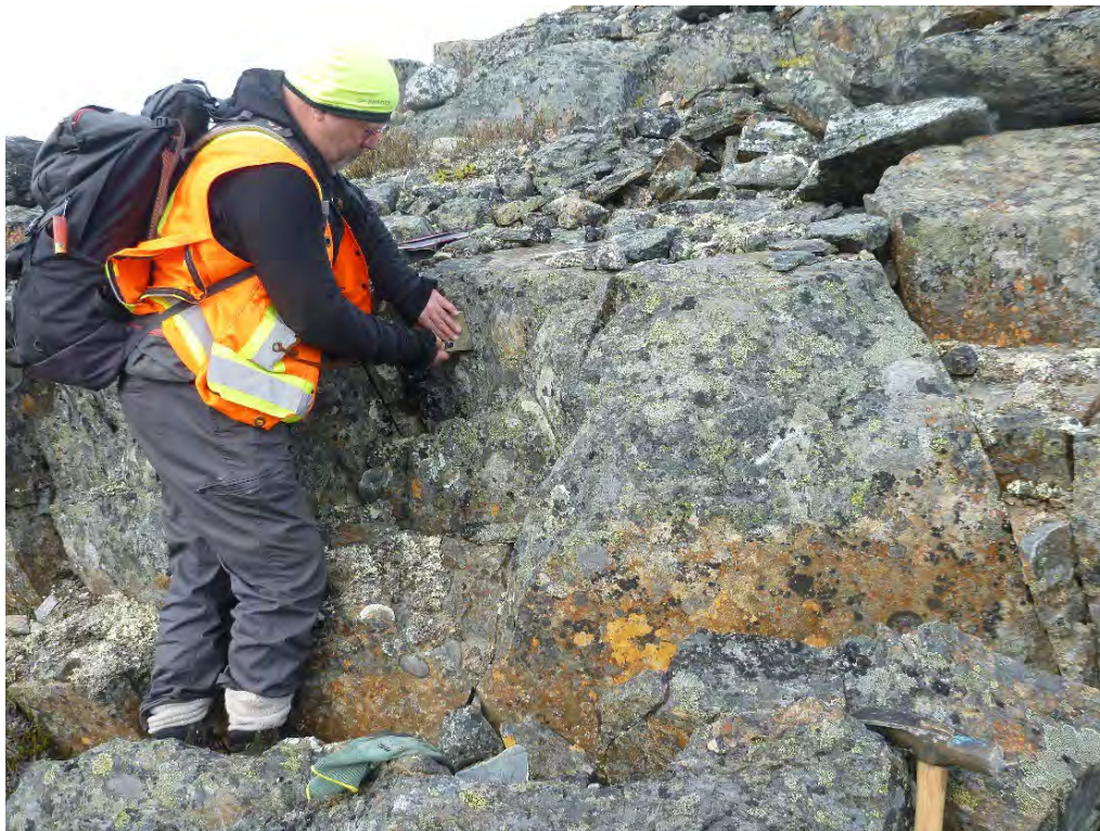
PHOTO 6 – Structural Geologist taking measurements with a Brunton
