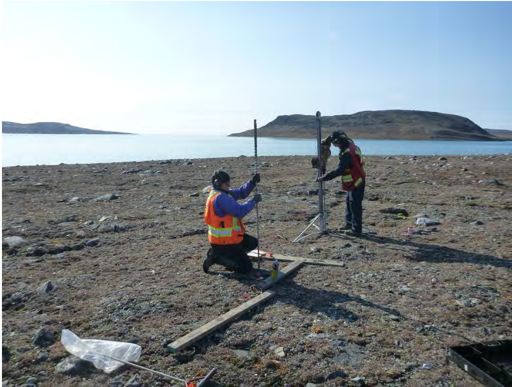
PHOTO 5 – Surficial Geologists using a talon drill to collect till and sediment
