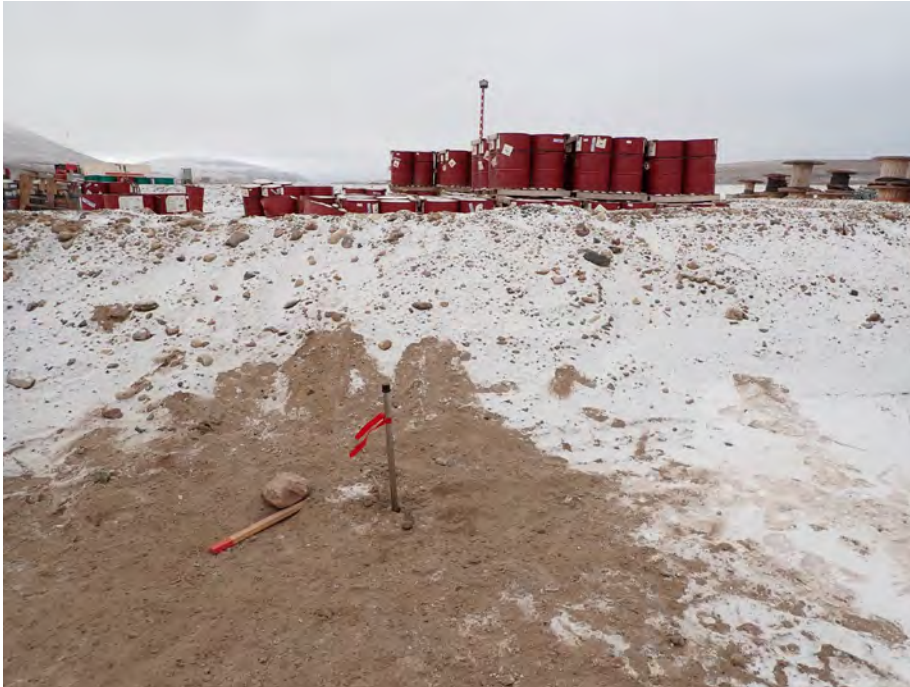
Photo 3: Drive-point piezometer installation - monitoring location MS-HWB-GW4, facing east-southeast. September 19, 2021
