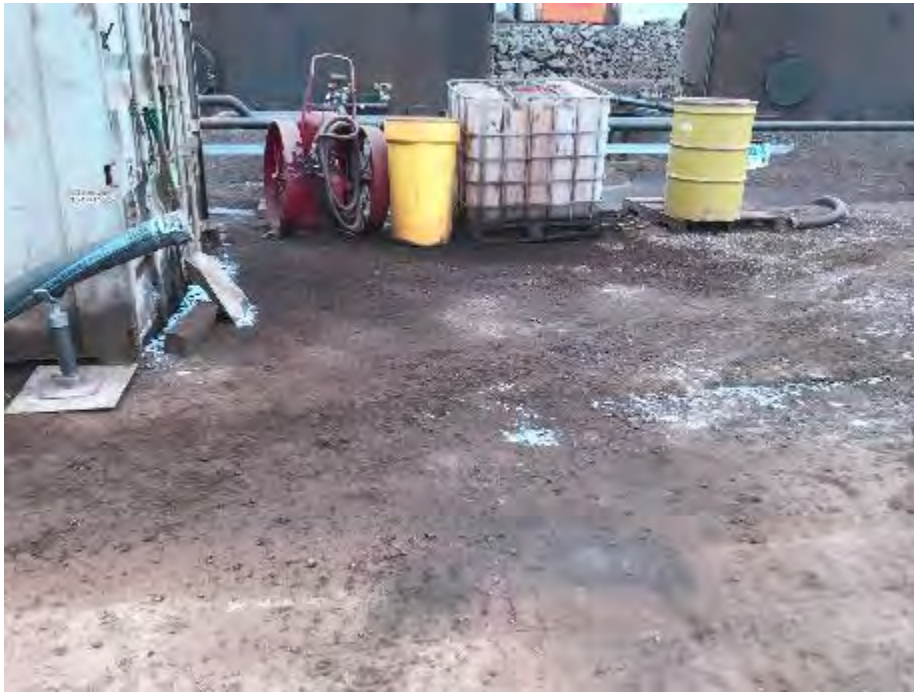
Photo 57: Site Reconnaissance at Fuel Farm MS03B, showing PHC staining on the surface. September 27, 2021
