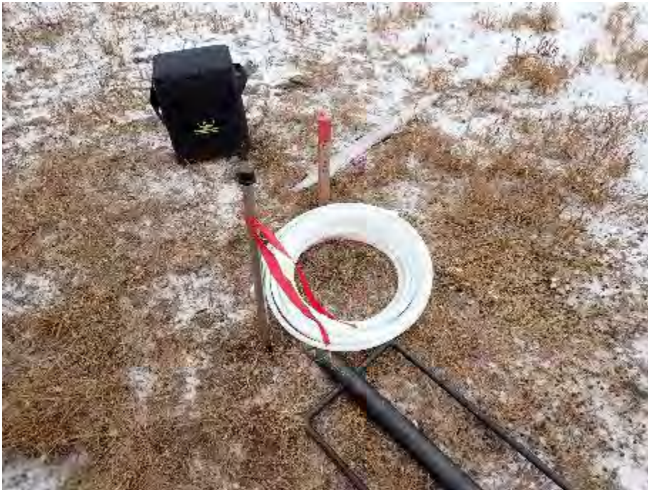
Photo 6: Drive-point piezometer installation - monitoring location MS-HWB-REF2. September 19, 2021
