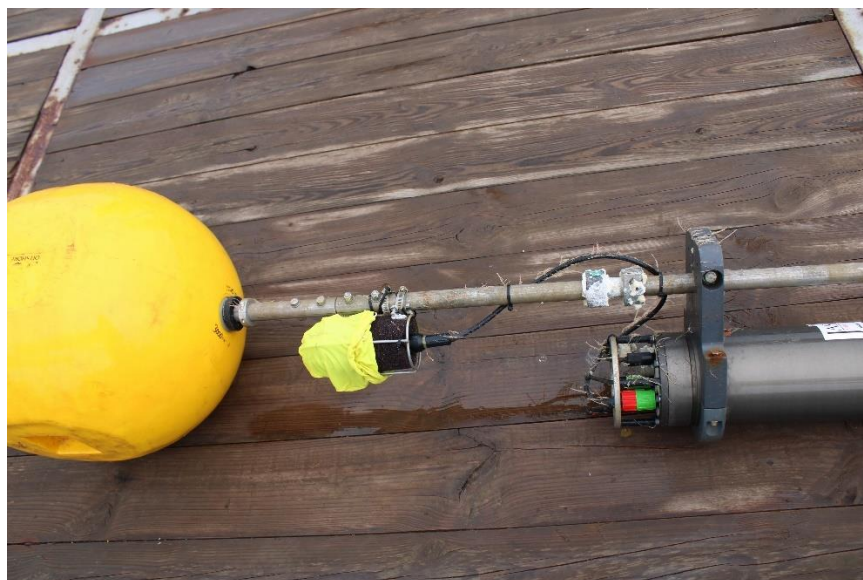
Figure 5. Configuration of AMAR-WFE and AMAR-EFE showing hydrophone location.
