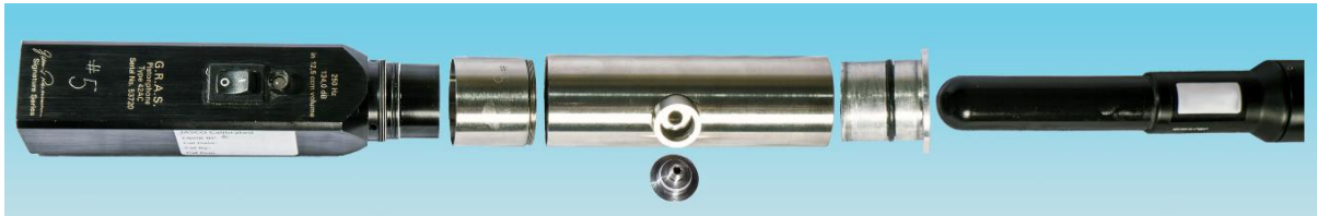
Figure A-1. Split view of a G.R.A.S. 42AC pistonphone calibrator with an M36 hydrophone.
