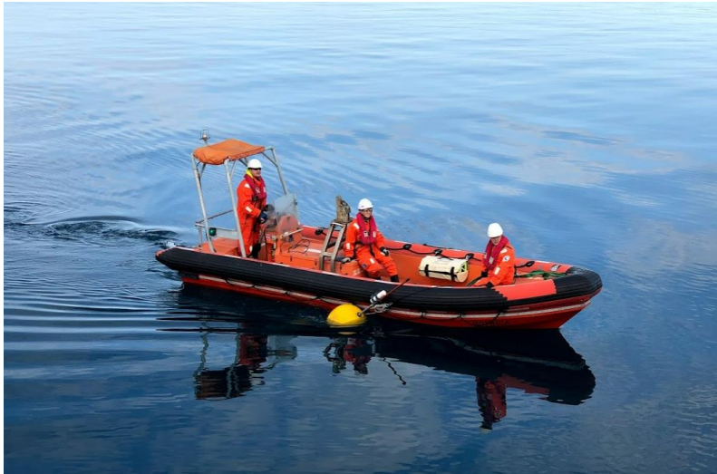
Figure 8. The fast rescue craft from the MVS Botnica towing the AMAR mooring to the vessel post retrieval.
