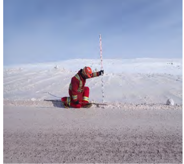
Photo 10-6. Compliant snowbank (9cm) at KM 55 with signs of snowbank management (feathering) on April 19, 2022.
