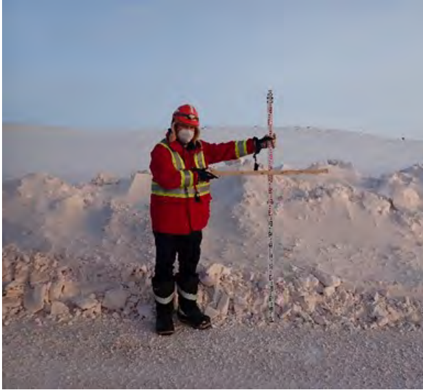
Photo 10-5. Non-compliant snowbank (138cm) at KM 93 (February 14, 2022).
