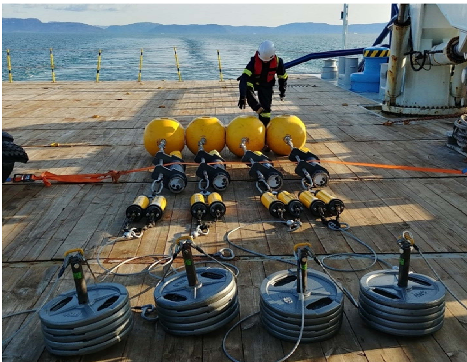
Figure 4. The Autonomous Multichannel Acoustic Recorder (in the middle of the mooring-AMAR G3; JASCO) used to measure underwater sound in and near Milne Inlet (North and South) and in Eclipse Sound.
