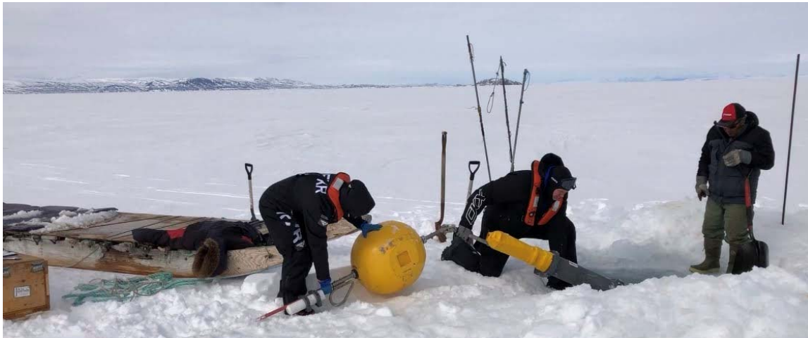
Figure 5. Through-ice AMAR deployment in Eclipse Sound in May 2019, supported by Tagak Outfitters (Photo: Ben Widdowson).
