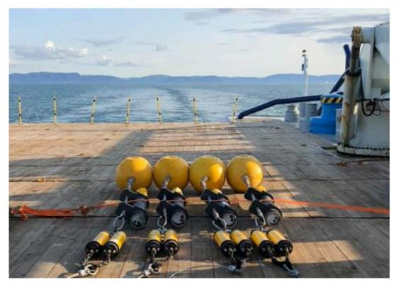
Photo 34: Acoustic Equipment was Deployed During Summer 2019 to Measure Underwater Noise
