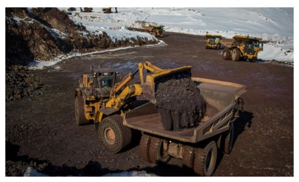
Photo 2: Iron Ore Being Loaded onto Mine Haul Trucks
