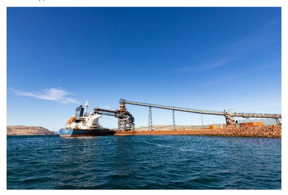
Photo 5: Vessel Being Loaded with Iron Ore at Milne Port using Ship Loading Conveyors
