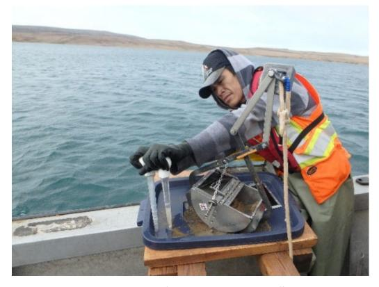
Photo 35: Benthic Grab Sampling as Part of the Marine Environmental Effects Monitoring Program
