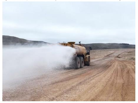
Photo 20: Dust Suppression Water Truck on Tote Road - August 2019
